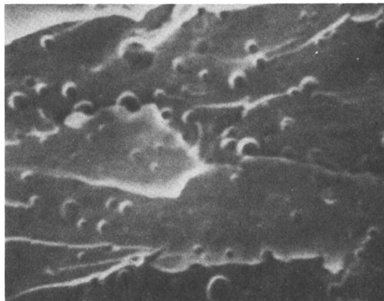
Figure 9. SEM of a fracture surface of an Epon 828–15% polar Viton GF blend. Magnification, 6,800 \times .
